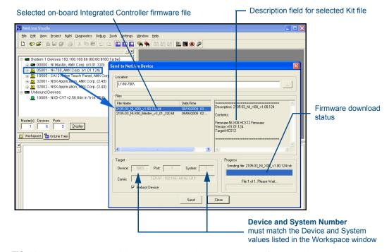
FIG. 31 Send to NetLinx Device dialog (showing on-board Integrated Controller firmware update via IP)
